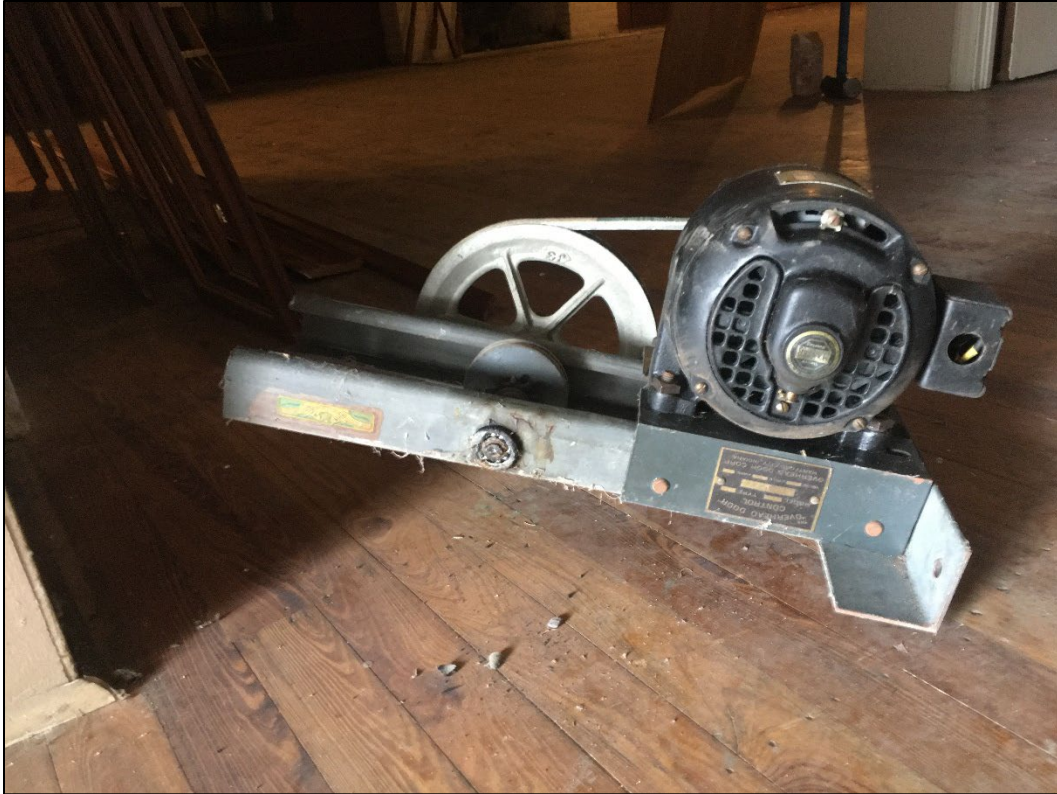
Figure 16. Salvaged garage door opener motor.
